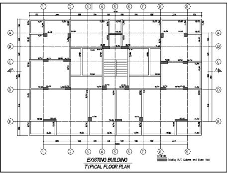
Figure 2. Typical structural as-built plan drawing
