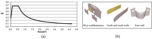
Figure 4 : Inelastic spectrum used in the analyses(a); Seperated walls for local analyses (b)
